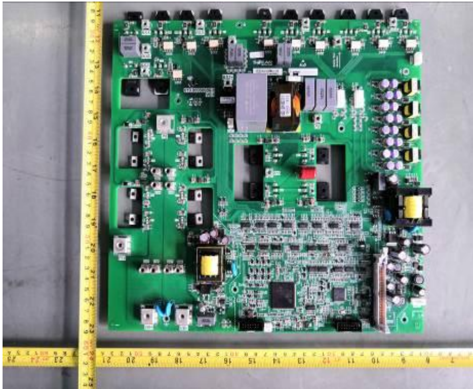
Power board view (Components side)
