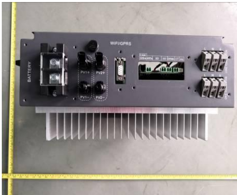
Connection terminal view
